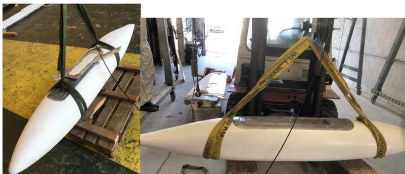
Section of the keel fin that is below the upper surface of the bulb
