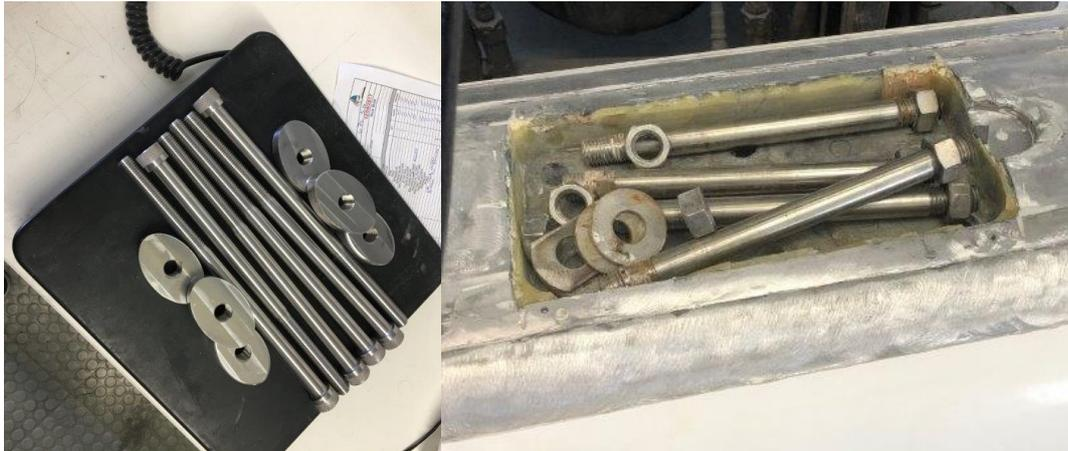
**A.8.1.2 Under-fin spacer plates that fit between the keel fin & bulb**
