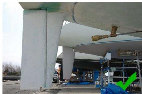
Skeg clearly visible as is propeller
