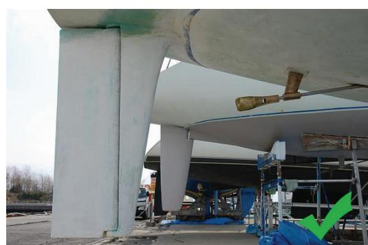
Skeg clearly visible as is propeller
